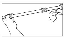
Loosen lower camlock and extend stem to desired operating length. Hand-tighten the camlock.
