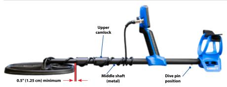
For submerged (diving) use, your *Vortex* can be collapsed as shown. Loosen the upper camlock and collapse middle shaft until pin locks into the position closest to the arm cuff.
